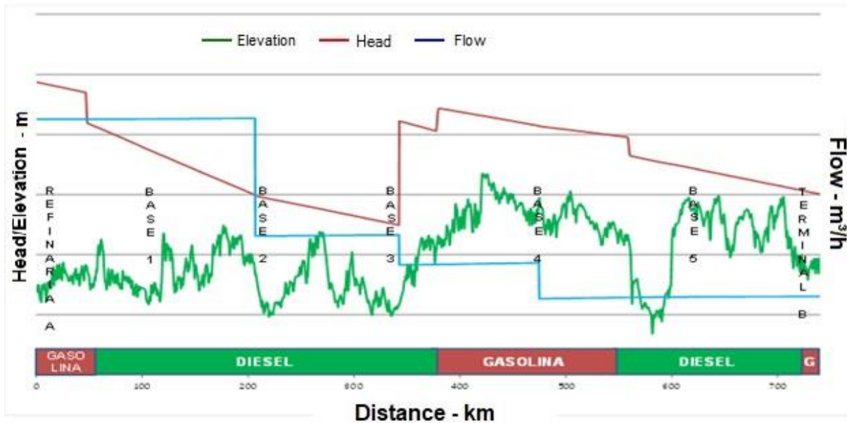
Figure 9. HEAD, ELEVATION, FLOW AND BATCHES POSITIONS WITH DRA ON OCTOBER 1ST
